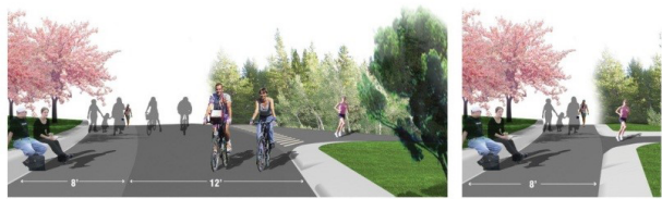
The new 20-foot-wide paths on the south Island are composed of an eight-foot-wide pedestrian walkway and a 12-foot-wide shared bicycle and tram lane. Pedestrian-only paths on the south Island are eight feet wide.
